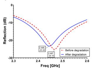
Fig. 4. The |S11| of the on-body reader antenna
